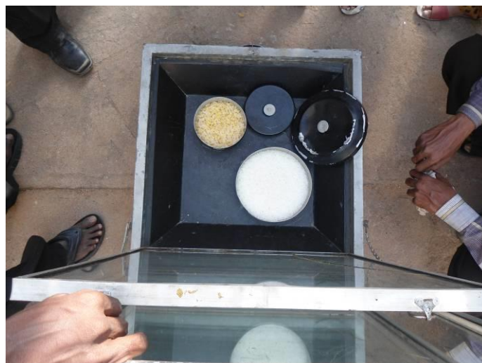
Evaluation and demonstration of Box type Solar cooker
