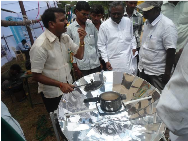
Evaluation and demonstration of Parabolic type Solar cooker
